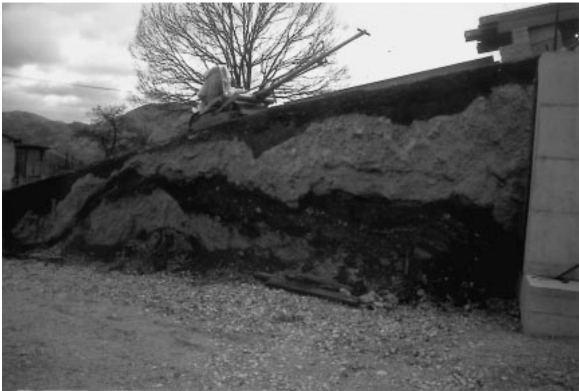
Fig. 6. Pergola site (sample PA3A): faulted debris slope deposits with interbedded palaeosoils (see text for details).
